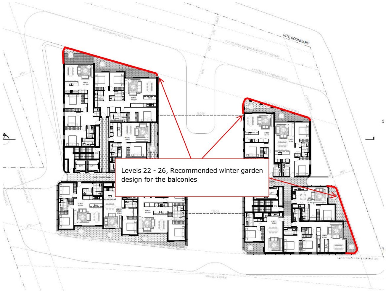
Figure 10: Recommended wind control measures for the large balcony on levels 22-26
